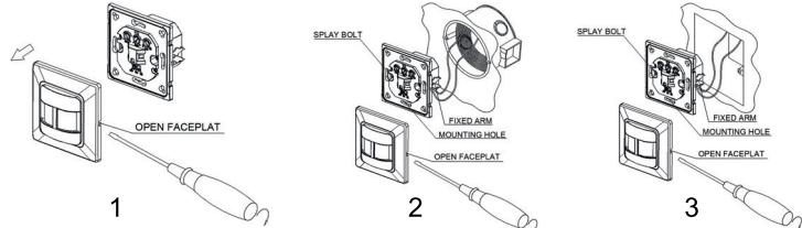
Unload the faceplate of sensor and adjust the time and LUX knob.(refer to 1)
