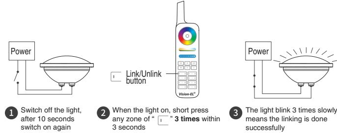
If the light not blink slowly, the linking failed, pls switch off the light again, and follow the above steps again.
