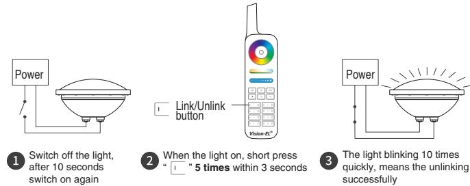
If the light not blink quickly, the unlink failed, pls switch off the light again, and follow the above steps to unlink again.
